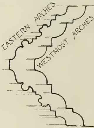
FIG. 1041. St. John the Baptist's, Perth. Section of Arch Mouldings in Choir and Nave.
